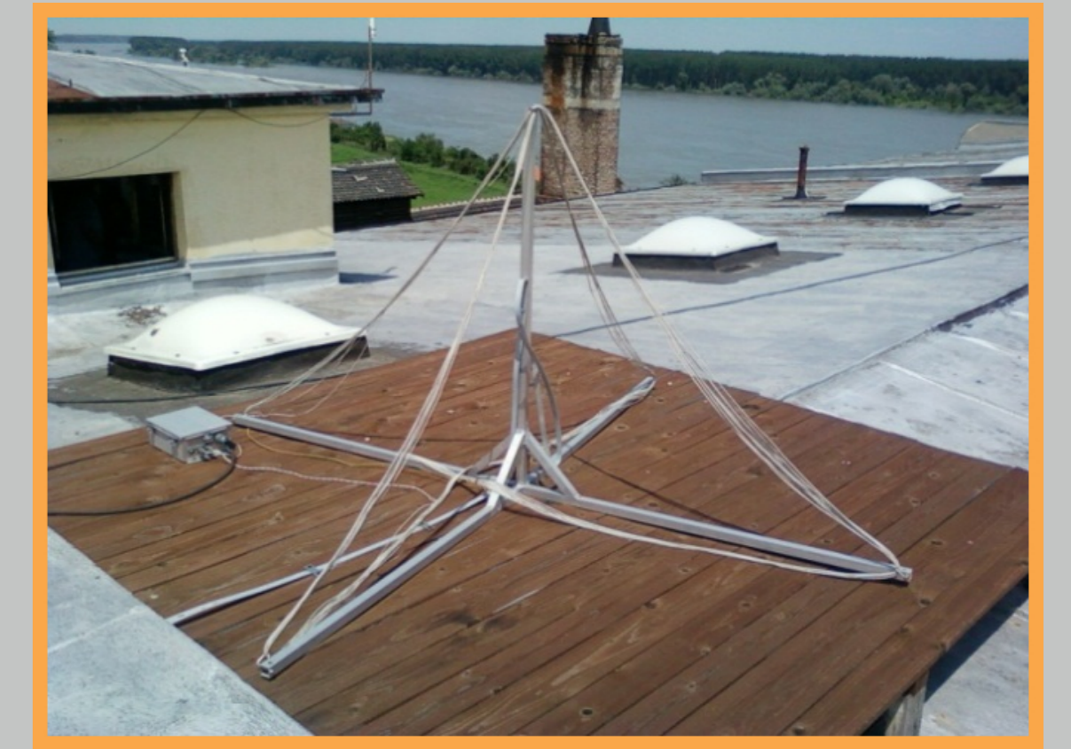
Belgrade ELF/VLF/LF Receiver Antenna
